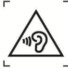
Figure 1 – Warning label (IEC 60417-6044)
