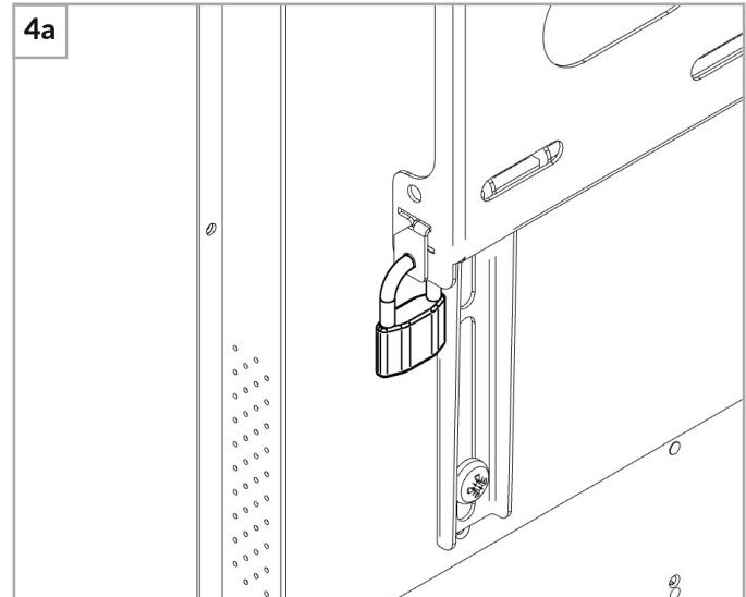
**EN** Pass the hasp of the padlock through the holes in the lock and the wall plate and close it.
