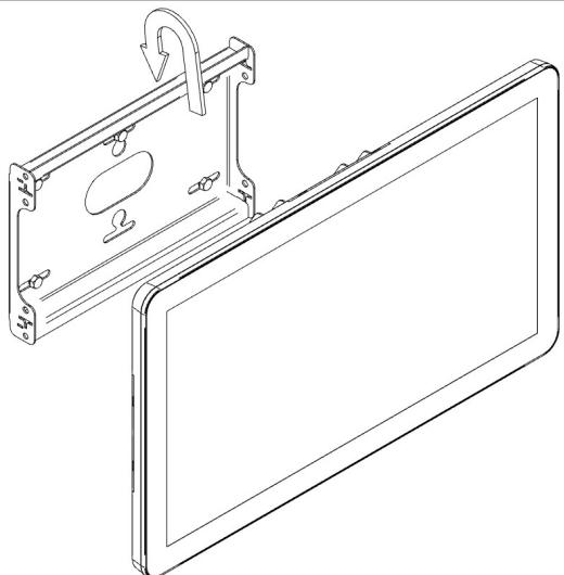
**EN** Hook the arms screwed to the monitor onto the wall plate.
