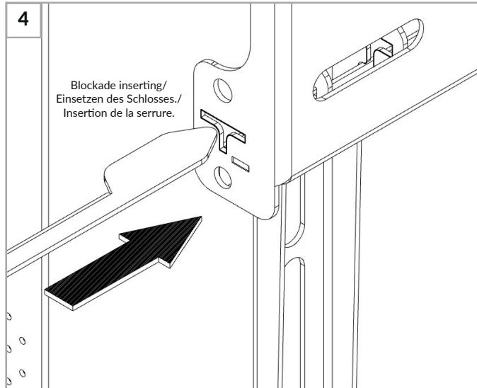
**EN** To protect the monitor against uncontrolled removal, secure it by inserting the lock into the "T" hole. The lock should go through the plate and both arms.
