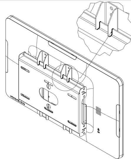
**EN** It should be noted that both hooks on both arms are hung on the board in a secure and stable manner.
