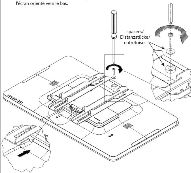
**EN** At this stage of assembly, connect all possible power and signal cables to the monitor.
