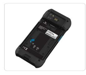
3 Insert the Micro SD card into the card slot.
