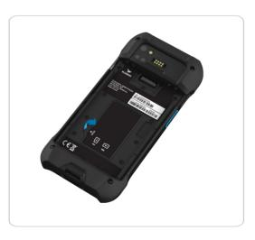
3 Insert the nano sim card into the card slot.
