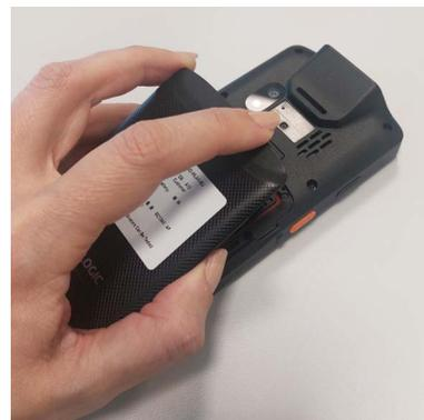
2. Insert the battery pack into the slot, top first, and press it into place.
