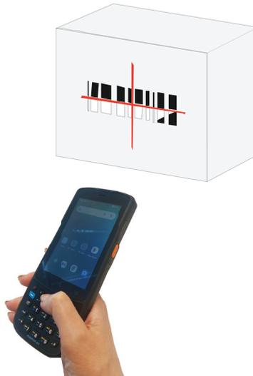
3. Center the symbol in any orientation within the aiming pattern. Ensure the entire symbol is within the rectangular area formed by the brackets in the aiming pattern, then either wait for the timeout or release the scan trigger to capture the image.
