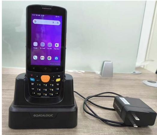
To remove the device from the dock, pull it upwards while holding the dock firmly down.
