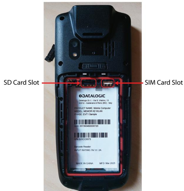
4. Replace the battery and the battery cover (see "Install the Battery" on page 7, steps 2 and 3).
