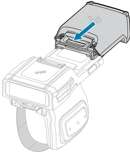
2. Slide the battery all the way into the locking slot.
