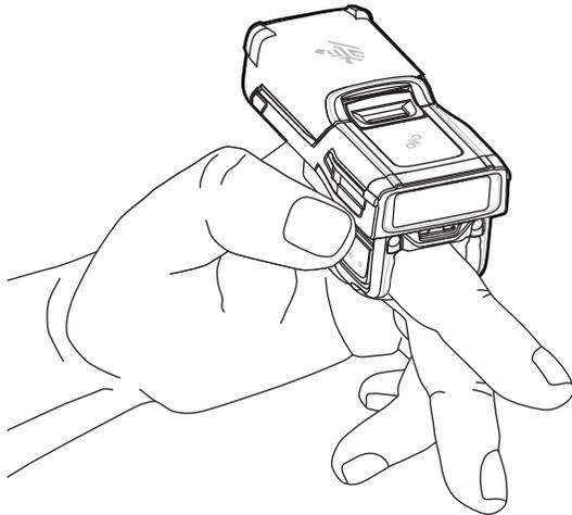
To tighten the finger strap on the single trigger, pull the end of the strap through the strap buckle. To loosen the finger strap, lift the strap buckle away from the strap while pulling the strap through the buckle. Release the buckle to hold the finger strap in place.
