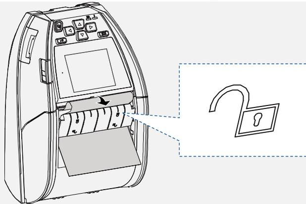
2. Feed the media go through the peeler module. (as figure shown)
