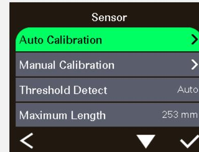
5. Press the **Menu** key to enter the LCD menu list. Go to [Sensor] → [Auto Calibration] to calibrate the media sensor.
