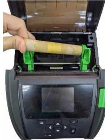
2. Release the lever. Install the label roll to stick the media holder.
