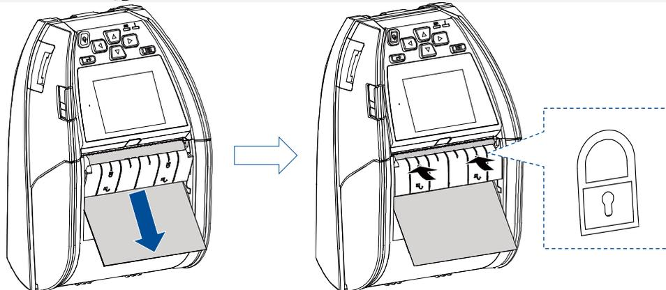
3. Pull the media tightly. Press down the peeler module to lock it.
