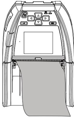
1. Please refer to section 3.3 to install the media and to calibrate the media sensor before loading media in peel-off mode.
