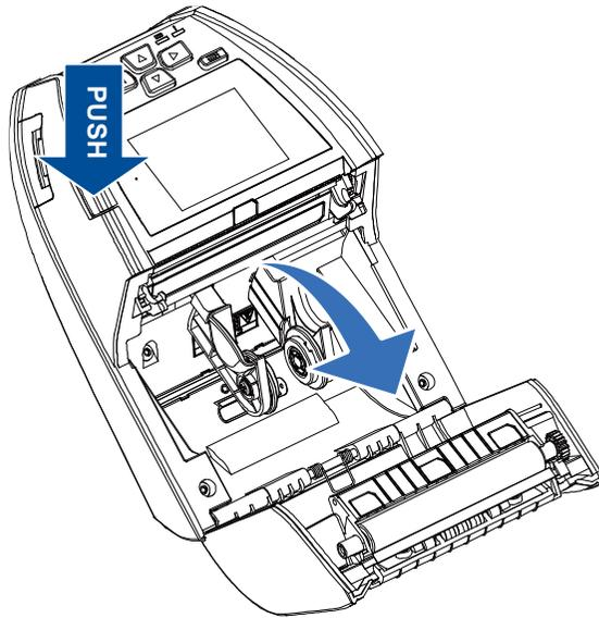
1. Open the printer media cover by pressing the media cover release button.
