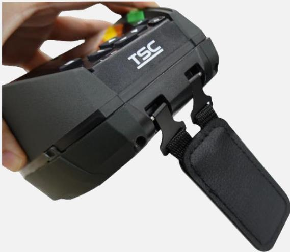
2. Press the hook of belt clip into the bars on the lower printer as pictured. The printer can be hung on the belt.
