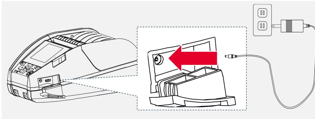
2. Plug the power cord to the power jack and power outlet.
