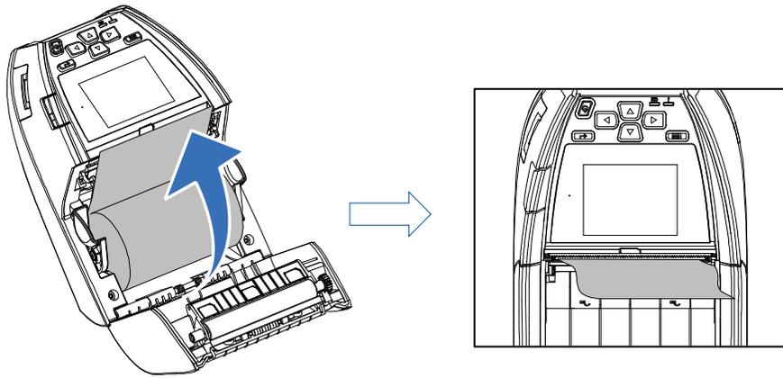
4. Press each side of media cover to close the media cover and make sure the media cover closed correctly.
