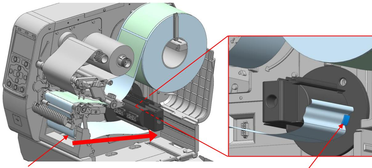
7) Adjust the rewriter fixing guides to the media width.
