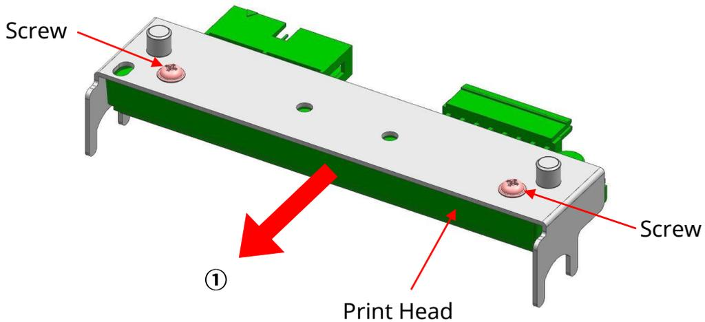
※ The factory default position of the print head (green side) is 0.6mm from the red guide in direction ②.
