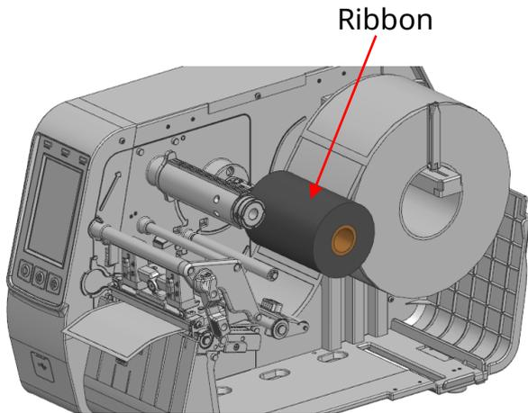
2) Open the print head lever and install the ribbon as shown below.
