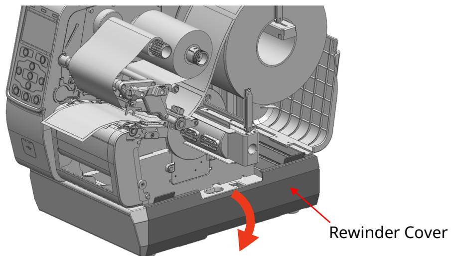
3) After flip down the rewinder fixing guide, install a 3inch media core on the rewinder holder.
