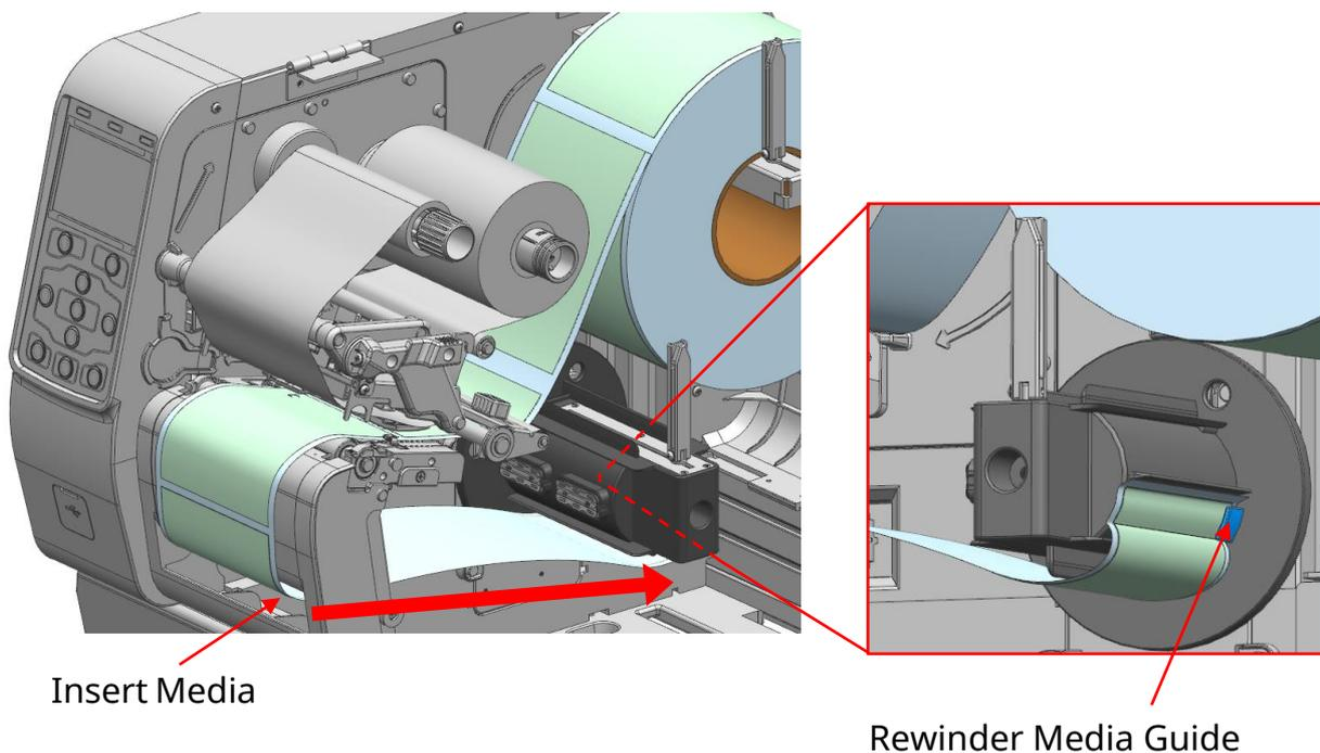
4) Adjust the rewriter fixing guides to the media width.
