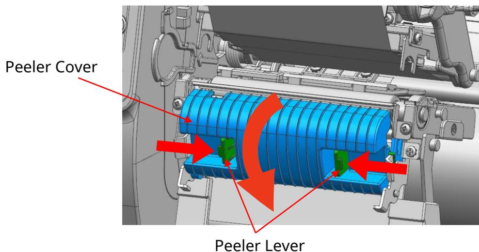
4) Move the peeler switch to ON. Please make sure that the LED has turned on.
