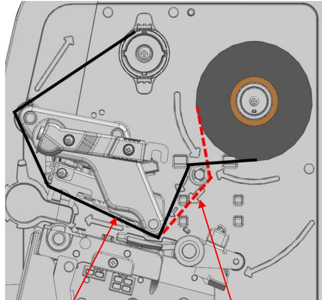
3) Attach the ribbon to the ribbon take-up spindle using tape.
