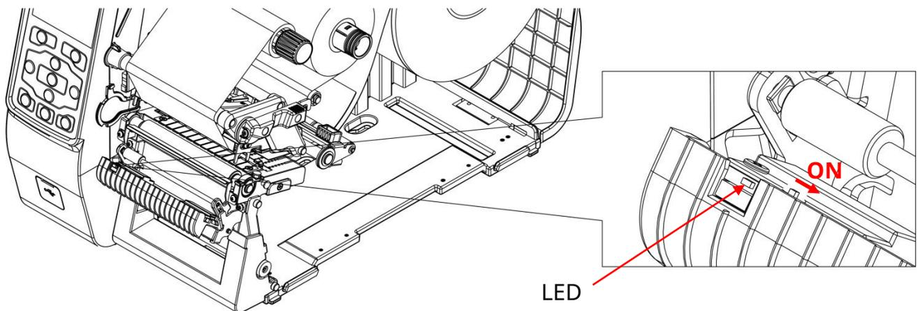
4) Remove several sheets of label media and insert liner as in the picture.
