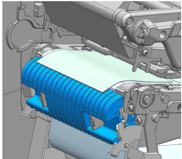
Peeler Sensor Be careful that the media does not cover the peeler sensor
