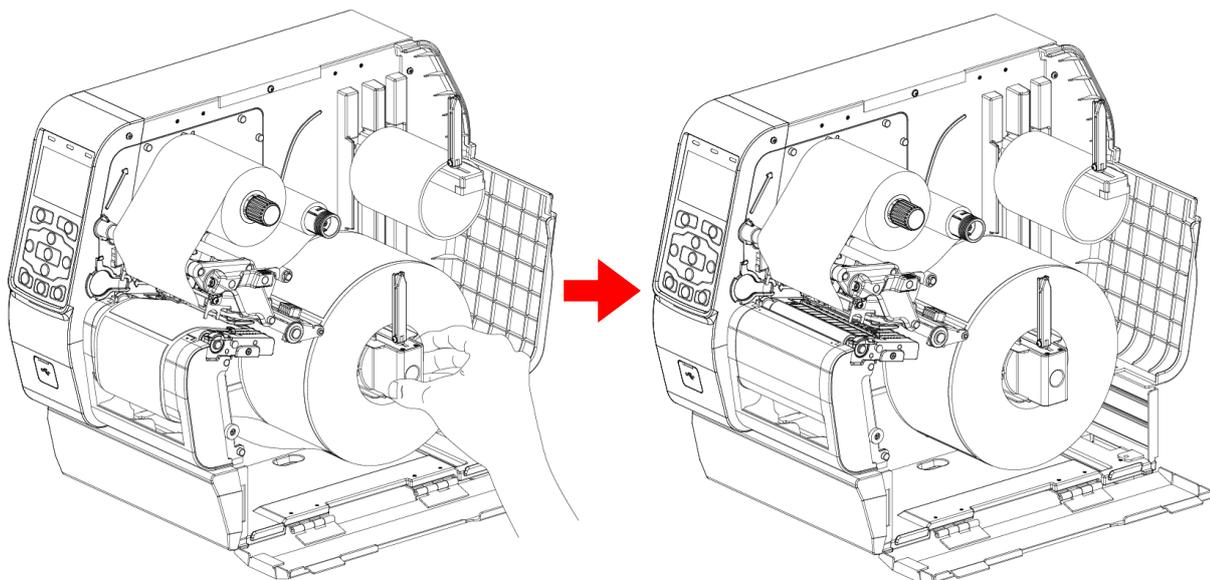
3) After flip down the rewriter fixing guide, push it inside.
