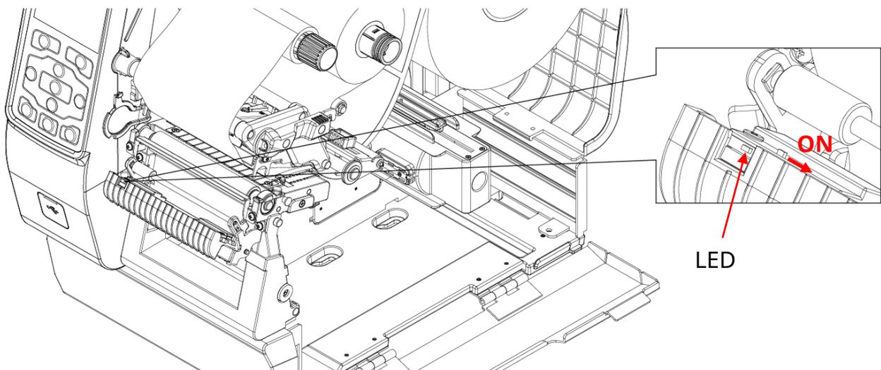
5) Remove several sheets of label media and insert liner as in the picture.
