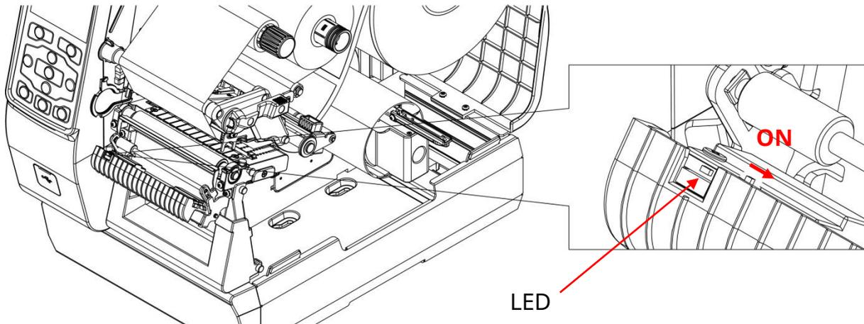
5) Remove several sheets of label media and insert liner as in the picture.
