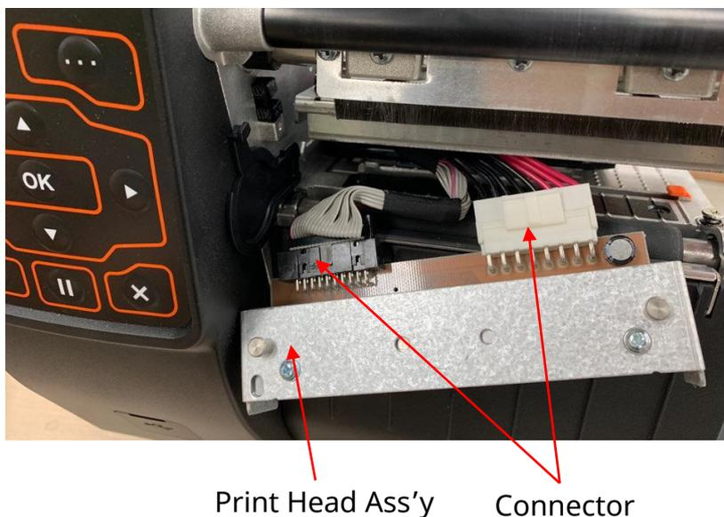
5) After loosening the screws using a cross-tip screwdriver, adjust the print head position.
