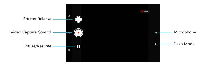
**Shutter Release** – Taking a picture while video recording is in progress.
