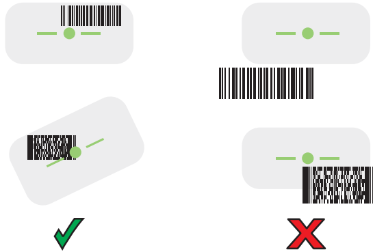
Figure 16 RS6100 Aiming Pattern
