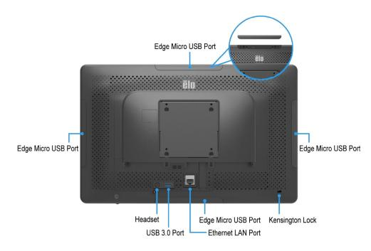
3 Make additional connections from the bottom of the stand module.
