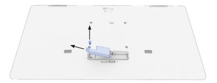
**2** Plug the USB-C cable from the I/O hub to the rear of the I-Series 4 Slate display.
