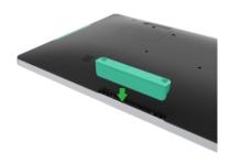
Gently insert the status light kit into the peripheral bay taking care to ensure the connector mates properly
