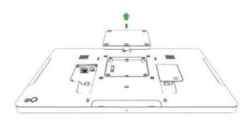
4 Secure adaptor to the I-Series 2.0 using 2 m3x16 screws (included)
