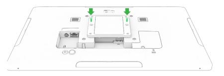
Optional 100x100 VESA spacer mounting: Place the spacer over the Elo POE module before adding VESA mounting bracket.
