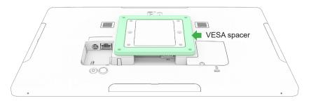
Attach wallmount or stand mounting brackets (not included) with screws long enough to pass through the POE module and into the threaded holes of the I-Series 4 VESA mount. Maximum screw depth is 5mm.
