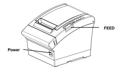
b. When booting process is complete, open the printer cover and press the FEED button for five seconds. The internal buzzer will sound five times and printer will be in WLAN selection mode. Mount the paper properly, close the cover, and check that the following information is printed.
