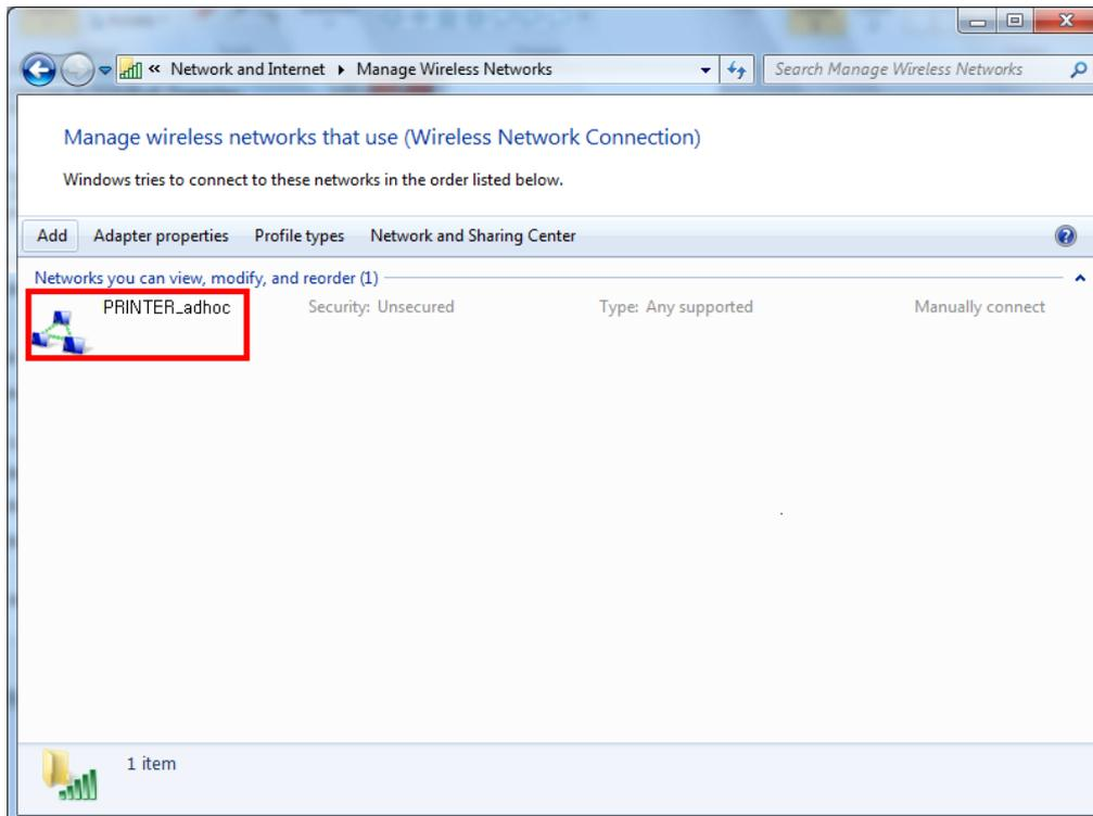
When the printer is set to the default value (Adhoc mode, SSID: PRINTER\_adhoc), it will automatically connect.
