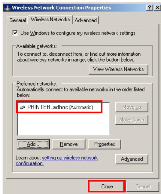
When the printer is set to the default value (Adhoc mode, SSID: PRINTER\_adhoc), it will automatically connect.
