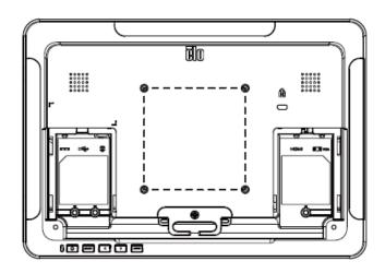
For the 1502L and 2002L touchmonitors, a four-hole 75x75mm and 100x100mm mounting pattern for M4 screws is provided on the rear of the monitor. Remove the stand using a Phillips screwdriver to access this mounting interface. The VESA FDMI-compliant counting is coded: VESA MIS-B, 75, C and VESA MIS-B, 100, C.
