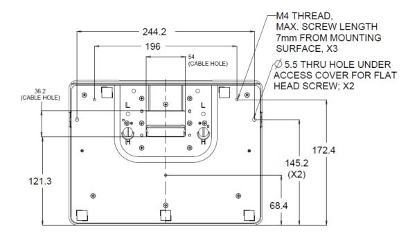
For the 2002L touchmonitor, threaded through-holes are provided on the bottom of the stand base for mounting or securing.
