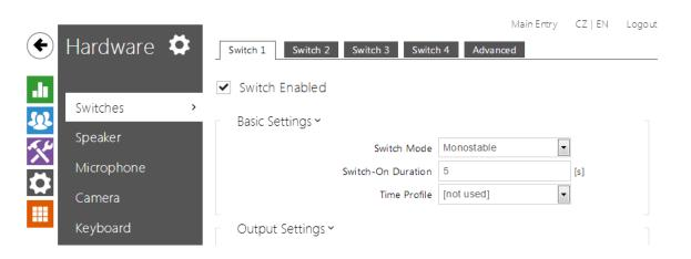
Switches provide a very flexible and efficient control of such intercom peripherals as electric door locks, lighting, additional ringing signalling, and so on.  $2N^{\ensuremath{\mathbb{R}}}$  Helios IP allo ws you to configure up to 4 (depending on model types) independent all-purpose switches.
