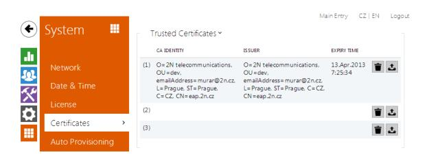
Some **2N**<sup>®</sup> **Helios IP** network services use the Transaction Layer Security (TLS) protocol for communication with other LAN devices to prevent third parties from monitoring and/or modifying the communication contents. Unilateral or bilateral authentication based on certificates and private keys is needed for establishing connections via TLS.
