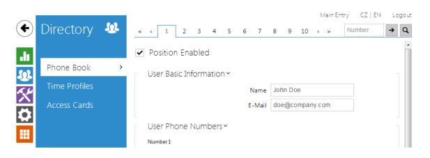
The Users list is one of the crucial parts of the intercom configuration. It contains user information relevant for such intercom functions as quick dialling, RFID card/code door unlocking, missed call e-mails and so on.
