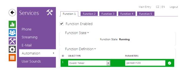
The  $2N^{\textcircled{B}}$  Helios IP intercom provides highly flexible setting options to satisfy variable user needs. There are situations in which the standard configuration settings (switch or call modes, e.g.) are insufficient and so  $2N^{\textcircled{B}}$  Helios IP offers  $2N^{\textcircled{B}}$  Helios IP Automation, a special programmable interface for applications that require complex interconnections with third party systems.
