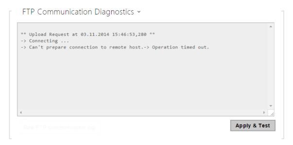
Click **Apply & Test** to save the current FTP server configuration, load the camera image and save the image to the FTP server. The window above displays the FTP server communication details during saving.
