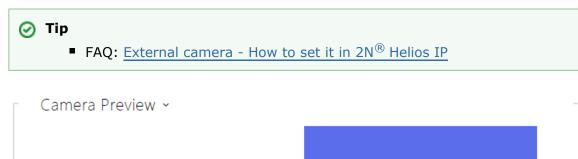
The Camera Preview window displays the current image received from an external camera. If the external camera is disconnected or configured incorrectly, the N/A characters are displayed on a blue background.
