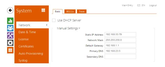
As the **2N<sup>®</sup> Helios IP** intercom is connected to the LAN, make sure that its IP address has been set correctly or obtained from the LAN DHCP server. Configure the IP address and DHCP in the **Network** subsection.
