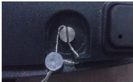
Locked with Wire Seal
