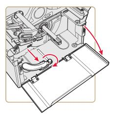
Raise the media roll guide to the upright position and insert the cardboard core onto the media roll rewinder hub.
