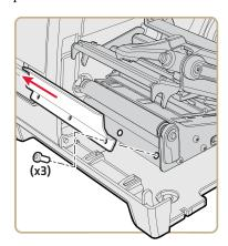
**3** Remove the five screws that attach the printer spine to the base.
