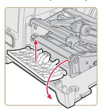
**2** Remove the three screws that connect the tear bar to the printer and remove it.
