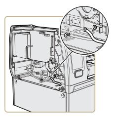
Feed the full roll rewinder cable through the cable clip and then insert it into the RWNDR connector on the main logic board.
