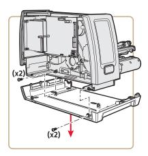
Remove Four Screws from the Electronics Side of Base
