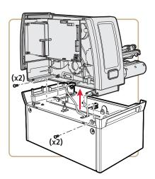
Attach the Spine with Four Screws on the Electronics Side
