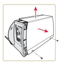
**3** Remove the electronics cover, and put the cover aside on a soft cloth to avoid scratches.
