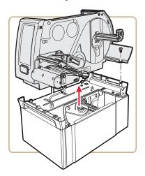
Attach the Spine with One Screw on the Media Side
