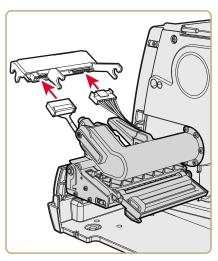
**7** As you insert the new printhead bracket into the printer, make sure the metal arms on the printhead go around the magnetic pressure arm bar. Attach the magnetic pressure arm to the printhead.
