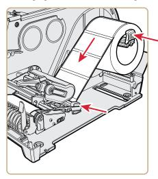
**5** Route the media through the print mechanism and out the front of the printer.
