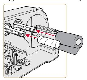
**4** For ribbon that has the ink wound out, place the ribbon on the supply hub with the ribbon wound clockwise. For ribbon that has the ink wound in, place the ribbon on the supply hub with the ribbon wound counterclockwise.
