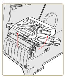
**3** Feed media through the slot in the back of the printer (or from the slot in the bottom of the printer) and route it through the print mechanism.
