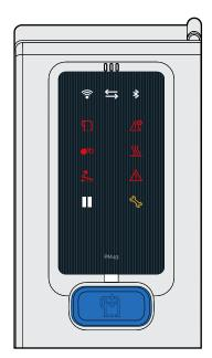
Icon Front Panel on a PM23c, PM43, and PM43c Printer
