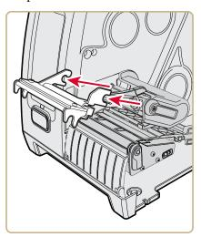
**6** Connect the two printhead cables to the new printhead.
