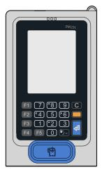
The Full Touch Display Front Panel on a PM43 and PM23c Printer
