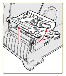
Load a media roll onto the media supply hub. Make sure you push the roll all the way against the inner wall of the printer and adjust the edge guide and the dancer guide to hold the media in place.
